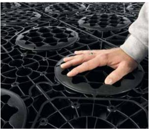
To ensure the geomembrane or geotextile can be wrapped around the tank snugly, covers should only be inserted in the top layer of the ACO StormBrixx® system. They prevent the geomembrane or geotextile being forced into the necks of the pillars during backfilling.
